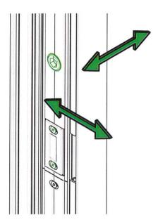
Keep - horizontal + 1 to 4mm: Using a 10mm Allen Key - 1/4 turn = 1mm, Full turn = 4mm
