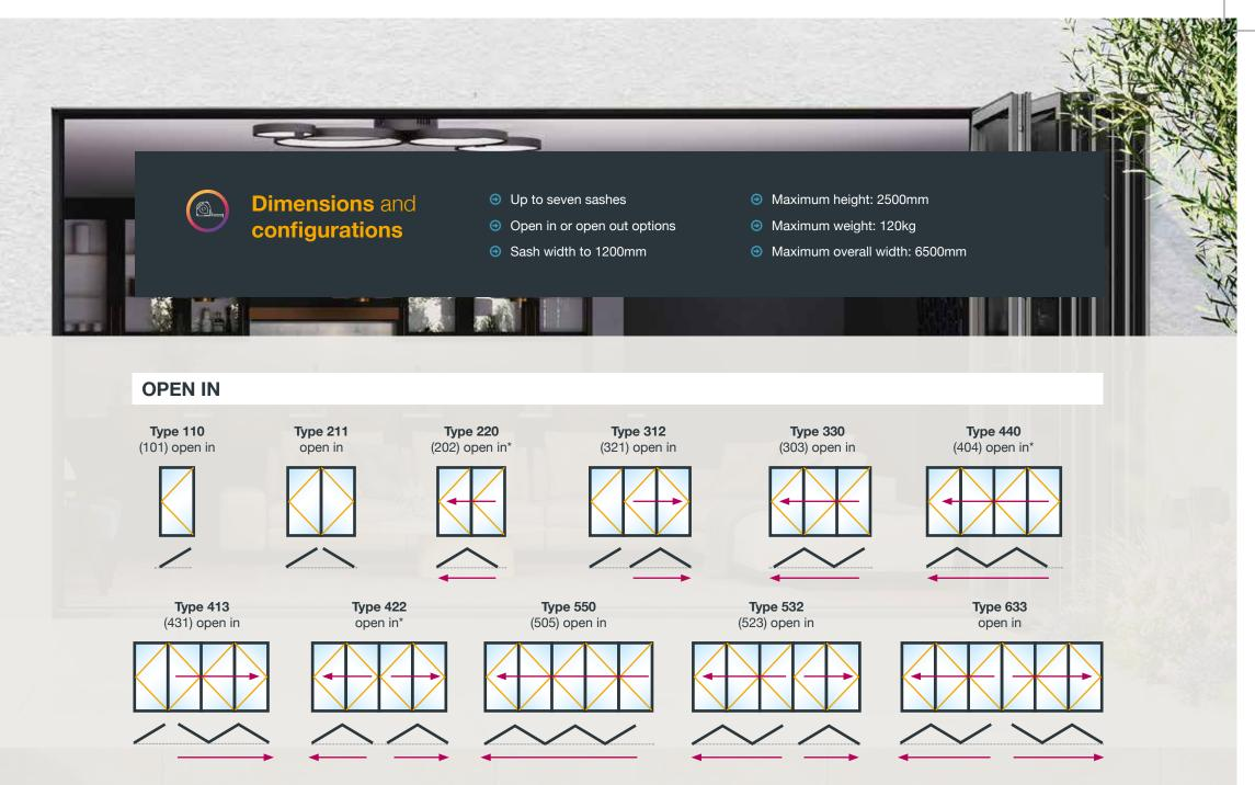
The most common configurations are shown above, but other styles featuring up to seven panes are also possible (please refer to the technical manual). \*No external access or traffic door with this design.
