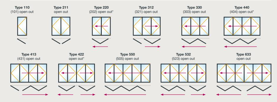
The most common configurations are shown above, but other styles featuring up to seven panes are also possible (please refer to the technical manual). \*No external access or traffic door with this design.
